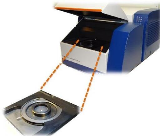
*Figure 5. Top panel:* optical components of NIR instrument to scan the sample in reflectance mode and *Bottom panel:* sample presentation in NIR device.
