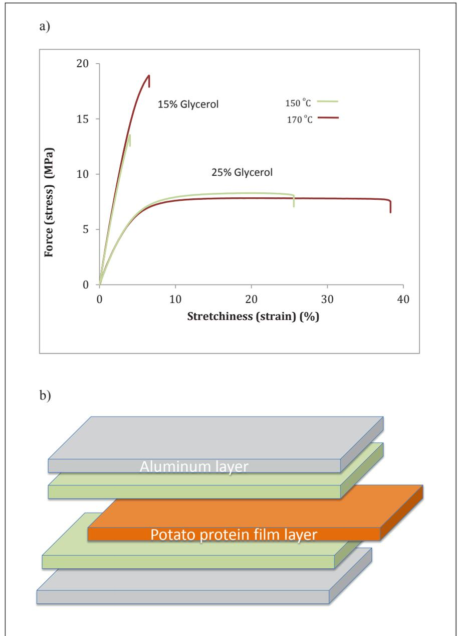
Figure 1 legend: a) Force (stress) and stretchiness (strain) for potato bioplastics formed with different amounts of plasticizer and at various processing temperatures, b) potato chip bag packaging example.
