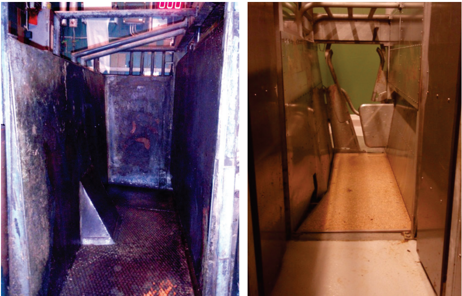
Figure 20. An outdated stun-box typical of older Swedish cattle abattoirs (left) compared with a more modern stun-box design conducive to improving cattle welfare (photos Sophie Atkinson).
