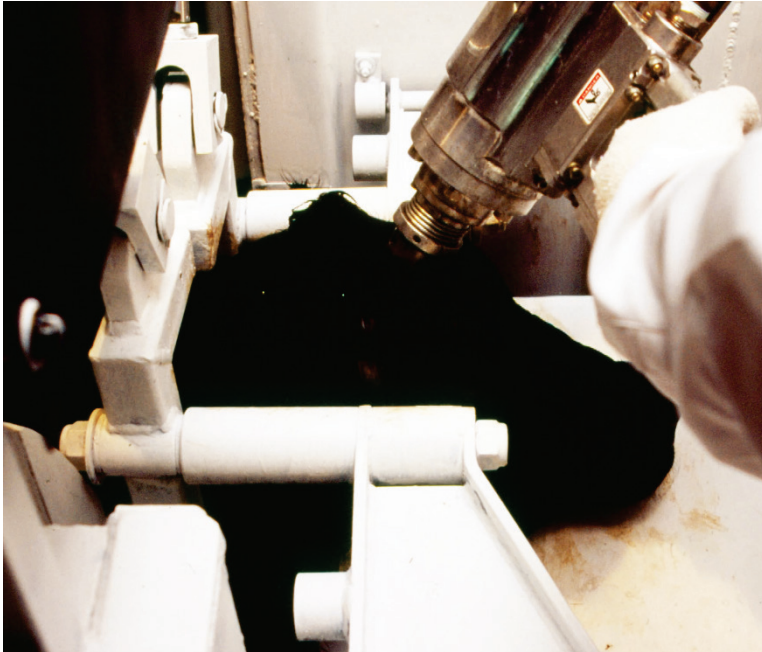
Figure 22. A relatively newer design of a highly restrictive head restraint in a stun-box used with a pneumatic stunner (photo supplied with kind permission from Jarvis).
