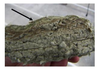
*Figure 2.* Cross-section of the upper layer of a slow filter consisting of compressed mineral wool granules. Filter skin samples were taken from the upper 5 mm of the filter column (indicated by arrow). Picture: Karl-Johan Bergstrand.
