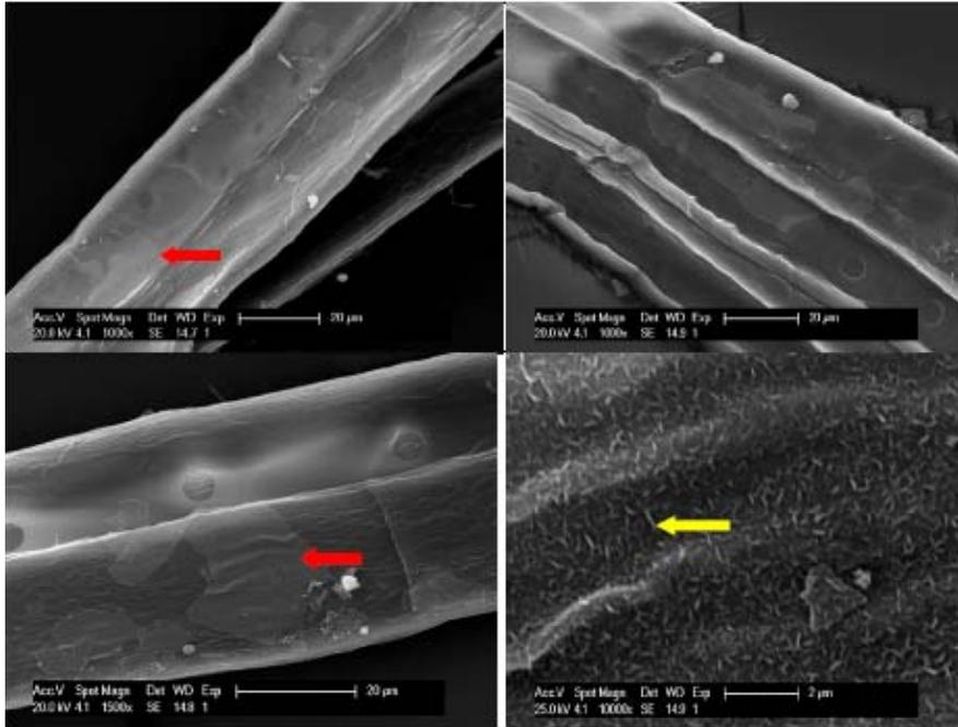
Figure 4a-b. Positive control; Reference-N; autoclaved with 10 g/L BX. Under these conditions the birch xylan can be observed forming isolated films on the fibre surfaces (arrows). Higher magnifications (bottom right) show these islands composed of fine flake-like structures (0.1-0.2  $\mu\text{m}$  long) that presumably represent concentrated xylan. Comparison of the images with Figure 12 shows indicates that the flake-like structures are embedded in a xylan film and may represent crystals.
