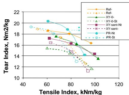
Figure 7b. Tear index vs tensile index for dried pulps.
