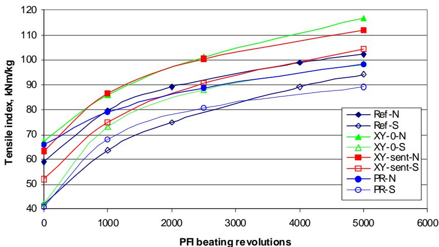
Figure 8. Tensile index vs PFI beating revolutions for never-dried pulps.
