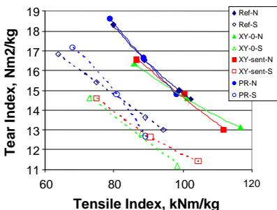
Figure 7a. Tear index vs tensile index for never-dried pulps.
