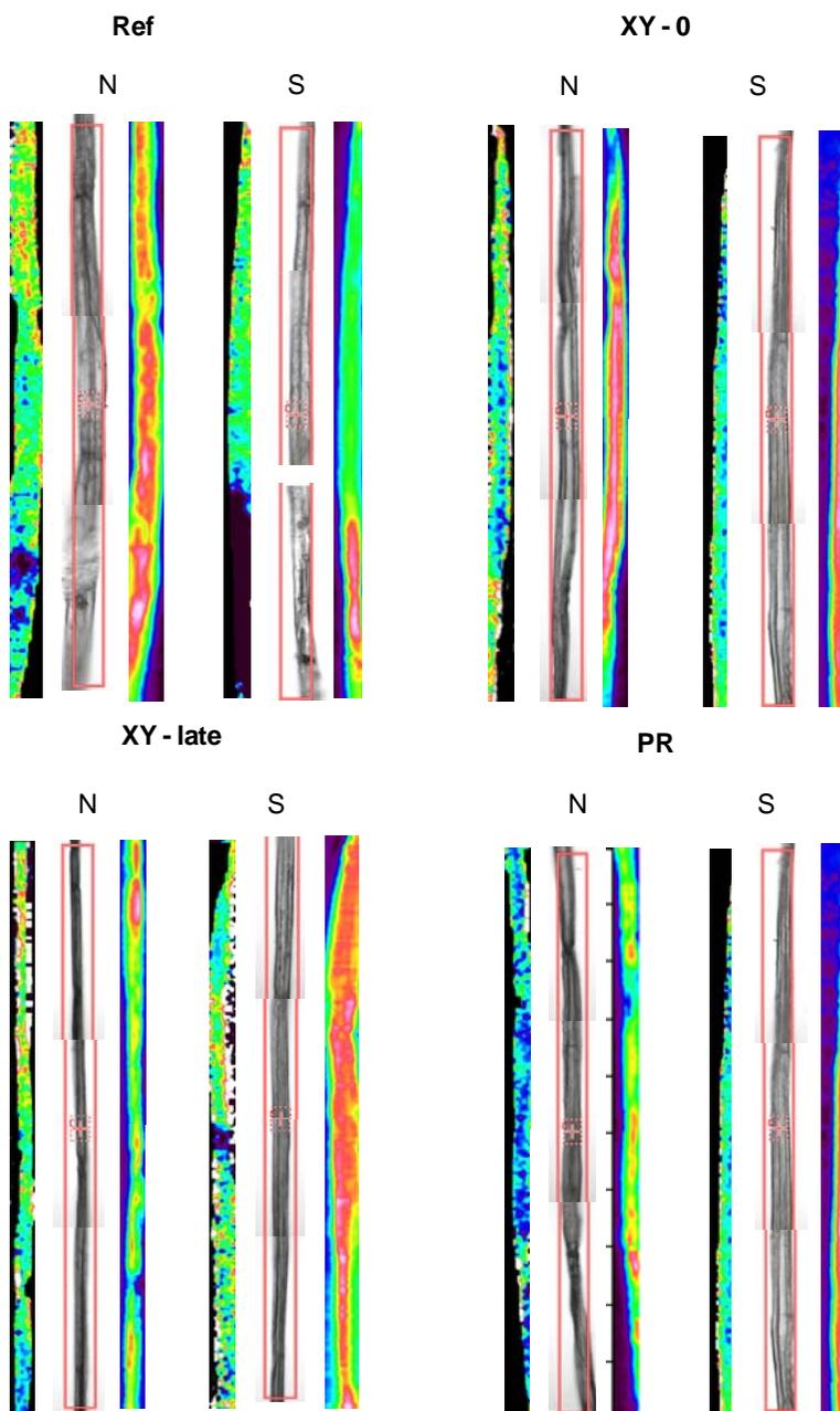
Figure 5. Images of 1 mm long sections of earlywood fibres of the 8 pulps. Each group shows from left to right: the xylan distribution image, i.e. the band ratio  $(1450-1460\text{ cm}^{-1})/(1360-1380\text{ cm}^{-1})$ , the microscopy image, and the total absorbance image.
