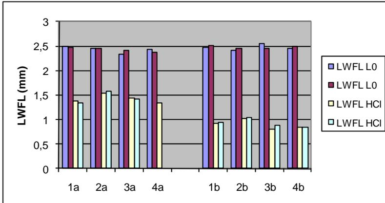
Figure 1. Fibre lengths of softwood pulp fibres before and after HCl treatment. Duplicate values. Normal fibres 1a-4a and sheared fibres 1b-4b as given in Table 1.
