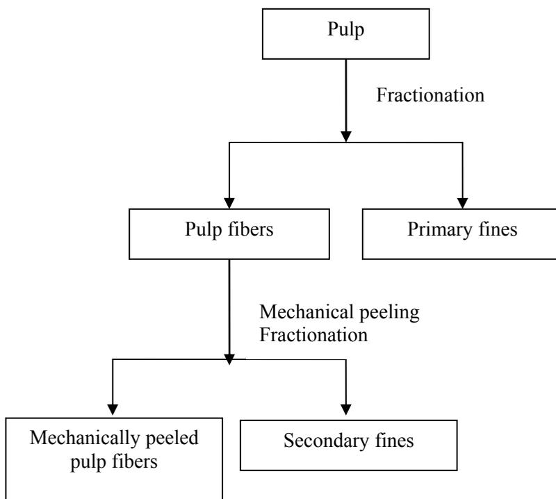
*Figure A1d. Procedure for mechanical peeling and fractionation.*
