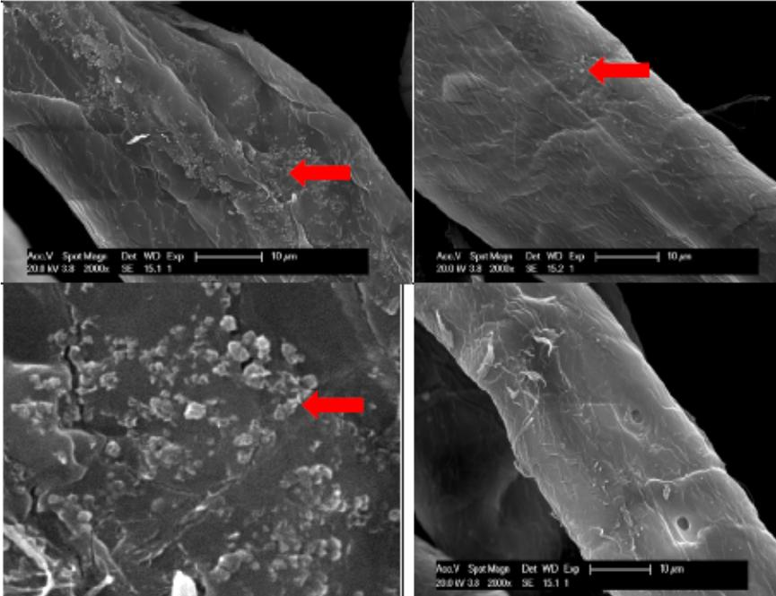
Figure 3a-d. Positive control; fully bleached pulp autoclaved with 10 g/L BX. Aggregates of birch xylan (arrows) present on areas of the outer fibre walls.
