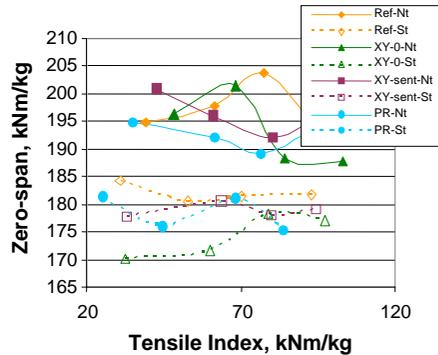
Figure 6b. Zero-span vs tensile index for dried pulps.
