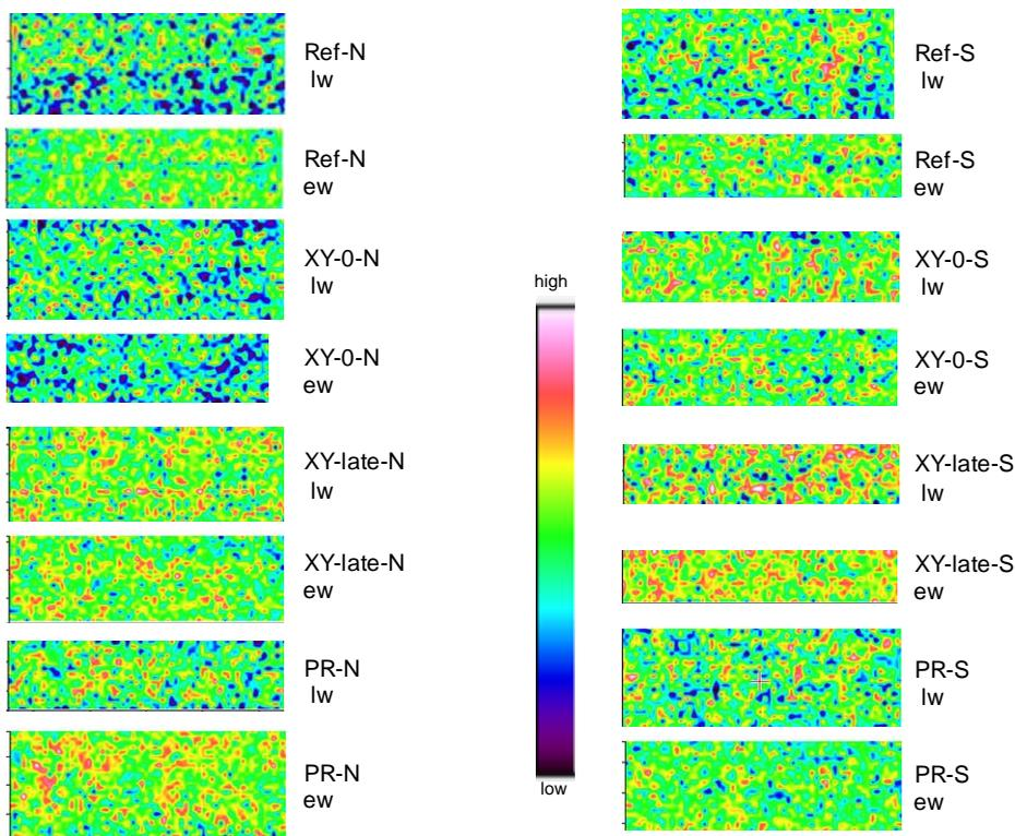
Figure 3. Intensity maps displaying the distribution of xylan on the fibre surface using the same scale for the different pulps. Red colour represents high amounts of xylan and black low amounts (lw=latewood, ew=earlywood).
