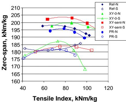
Figure 6a. Zero-span vs tensile index for never dried pulps.
