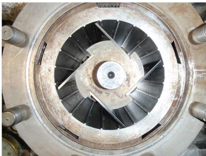
*Figure 2. Wing refiner at Aalto University in Helsinki.*
