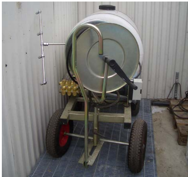
Fig. 7. Sprayer parking place on a permeable floor, above a sump pump pit, close to the pesticide storage
