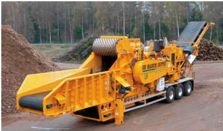
Figure 2. CBI Magnum Force 8400 horizontal hog with European chassis
