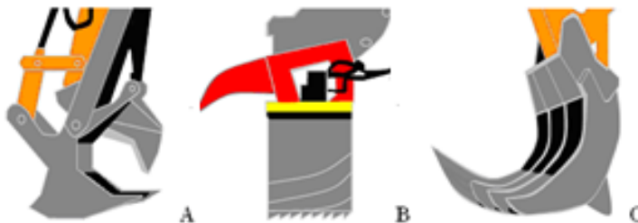
Figure 4. Stump harvesting heads used for extraction. A) Pallari, B) Rotary Cutter and C) Aalto.
