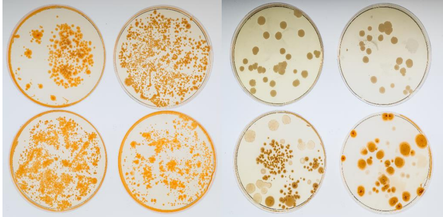
Figure 4.2. Photograph of plates from an attempt to do plate counting of colony forming units. The four plates on the left are control which have been cultivated without titania nanoparticles in LB-media. The four plates on the right were grown together with 50 mg/ml titania nanoparticles in LB-media.
