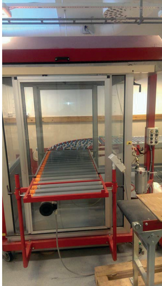
Figure 4. Ventilated spray chamber used for herbicide treatments in the experiment in Paper II.
