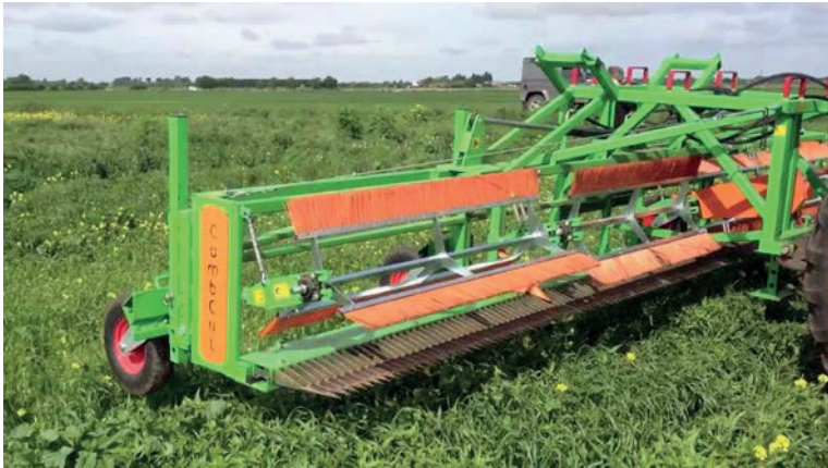
Figure 2. CombCut® machine, which selectively cuts C. arvensis and combs through the cereal crop without damaging it. Photo: Jonas Carlsson.
