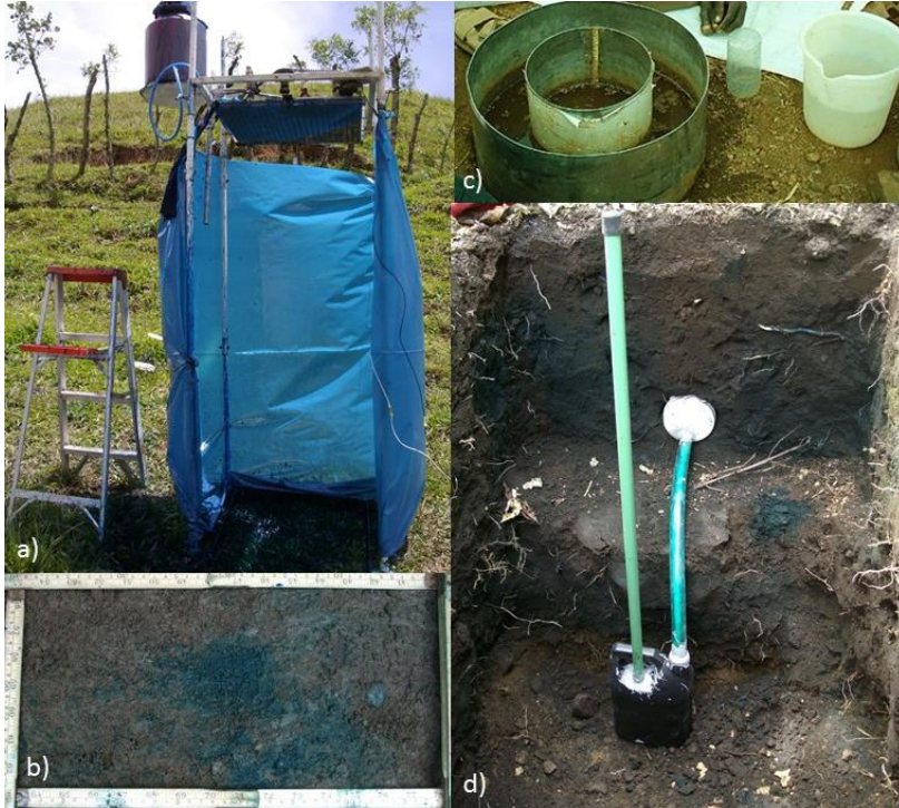
Figure 8. Main experimental methods to investigate the soil water dynamics: a) Rainfall Simulator; b) Frame of drying soil layer; c) Double ring infiltrometer; and d) Zero-tension wick lysimeter device.
