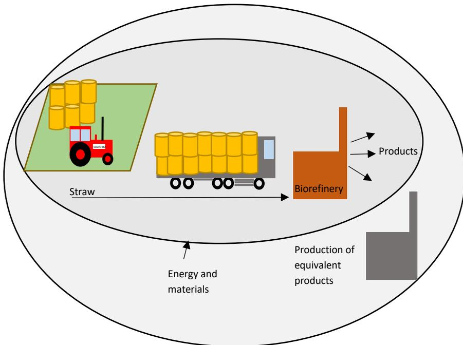
Figure 2. Illustration of the larger biorefinery system, including biomass production, harvesting and transport and effects on the surrounding system by substitution of equivalent products.
