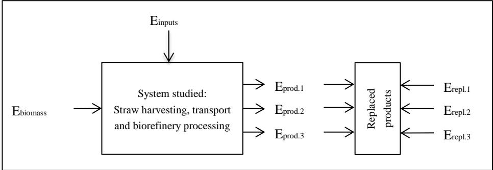
Figure 9. Variables for energy balance indicators used in Paper V.  $E_{\text{biomass}}$  and  $E_{\text{prod.1-3}}$  are given in lower heating value (LHV) and  $E_{\text{repl.1-3}}$  are given in primary fossil energy.
