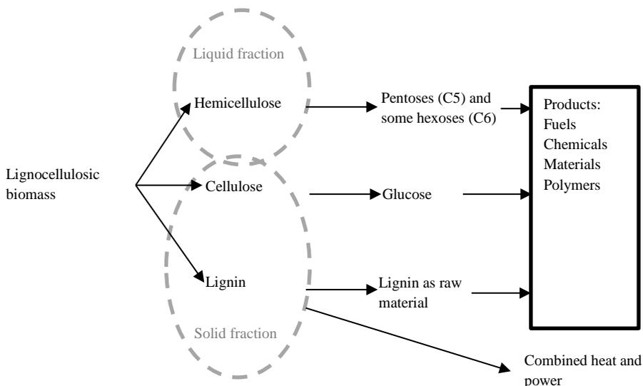
Figure 3. Schematic picture of a lignocellulosic biorefinery. The dotted circles represent the fractions after steam explosion as a pre-treatment (developed from Kamm & Kamm, 2007).
