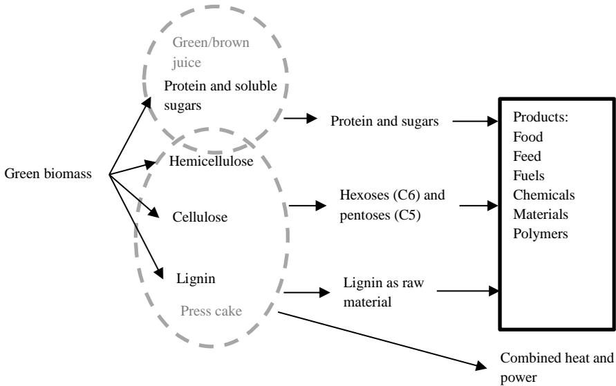
Figure 4. Schematic picture of a green biorefinery. The dotted circles represent the fractions after pressing the biomass (developed from Kamm & Kamm, 2007).
