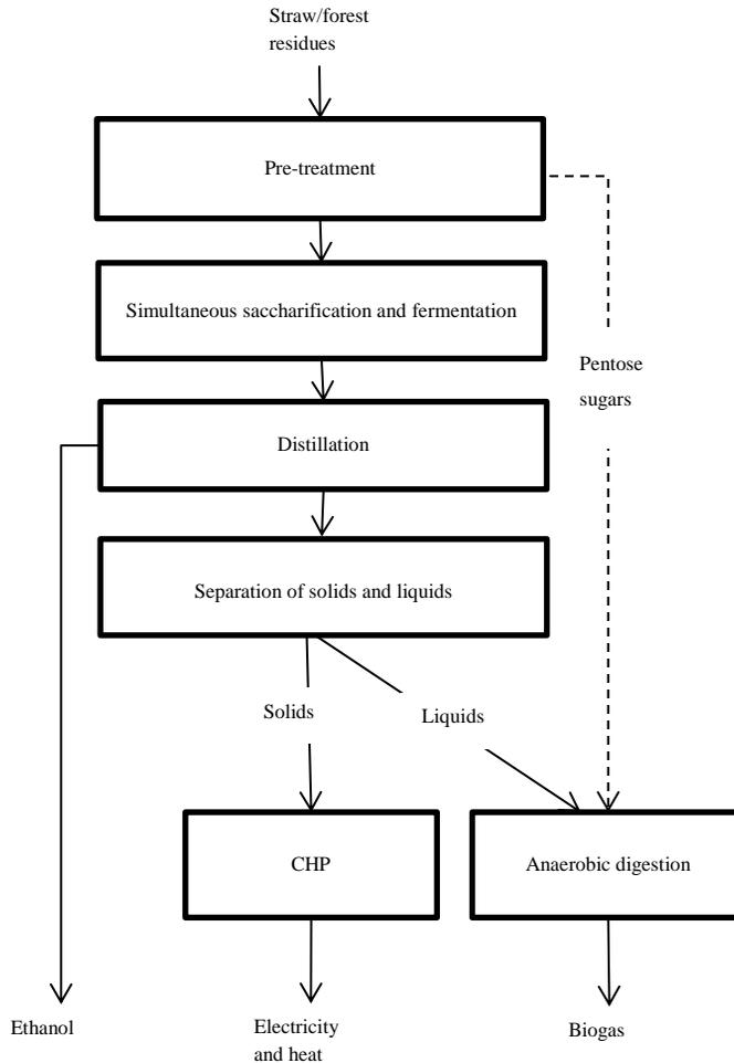
Figure 6. The biorefinery system considered in Paper II (modified from Börjesson *et al.*, 2013b). The dotted arrow represents feeding of pentose sugars from the pre-treatment directly to the anaerobic digestion (forest residue scenario) as opposed to all sugars going to the hydrolysis and fermentation (straw scenario).
