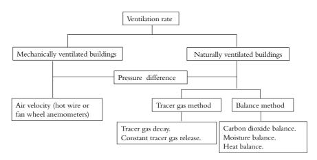
Figure 3. Methods for measuring ventilation rates in animal buildings
