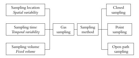
*Figure 2.* Factors and methods for gas sampling at animal facilities (adapted from Ni & Heber, 2008)
