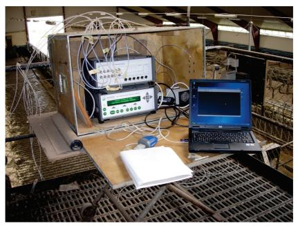
Figure 8. Photo-acoustic analyser coupled with a multiplexer during field measurements.
