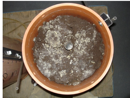
Figure 12. Gap between lysimeter wall and soil monolith after drying.
