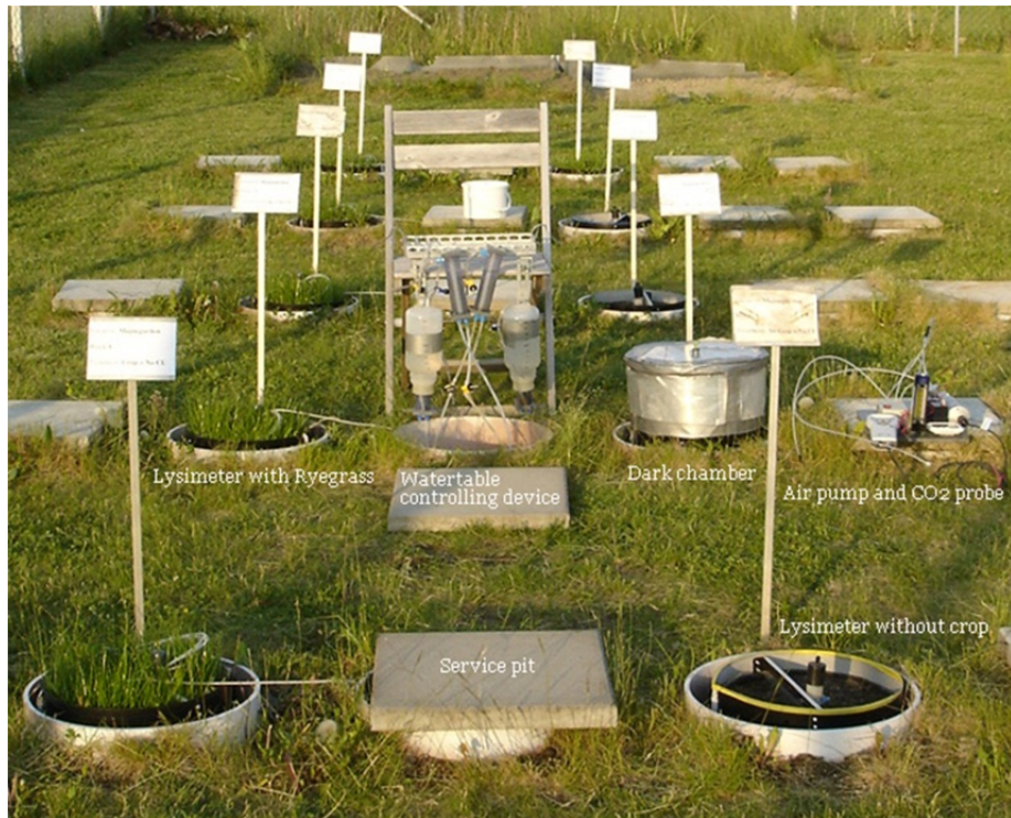
Figure 15. Lysimeter station used in the experiment. Service pits in the middle. The overflow device to control the water table is in a temporary elevated position in the second row. The dark chamber and the pumping device for gas sampling can be seen to the right.
