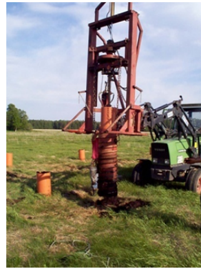
Figure 11. Soil monoliths collected with minimal disturbance in PVC casings.
