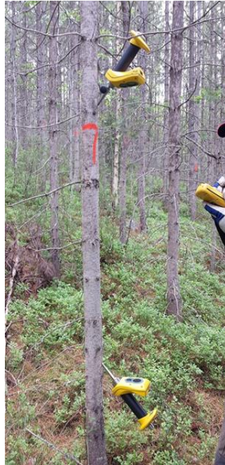
Figure 5. Hitman ST300 tool used to measure the acoustic velocity of standing trees
