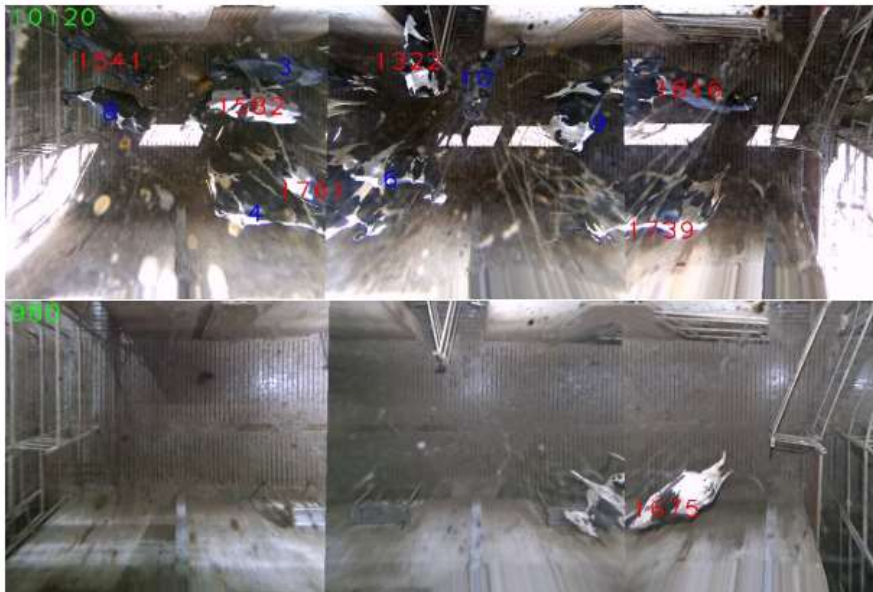
Figure 16. Example frames, with tracked objects marked, from the crowded, sunny (top) and easy (bottom) sequence. The red ID-numbers are initiated and assigned by the selection gates and placed on the correct cow by the tracker, while the blue numbers are placed manually in the first frame and then further tracked.
