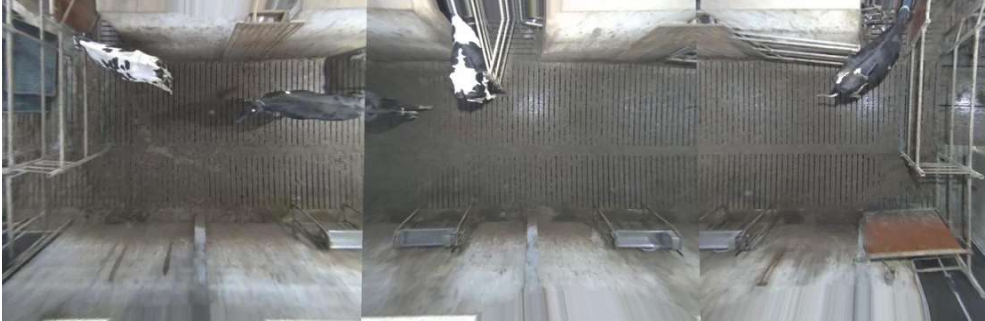
Figure 2. The frames from Figure 1 projected onto the cow shoulder plan and stitched together to form the overview over the entire waiting area.
