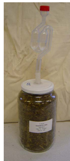
Figure 1. Type of lab silos used in our experiments.
