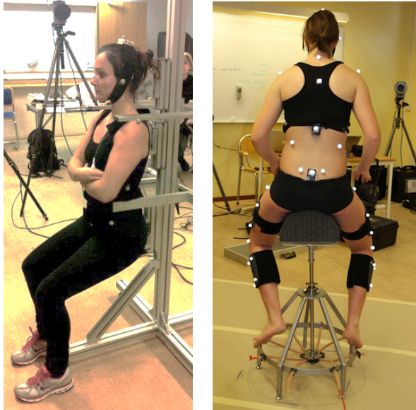
Figure 8: Stance chair (left) used to create stance files (marker tracking) and calibrate the IMU sensors. Balance chair (right), which was rocked from side to side.
