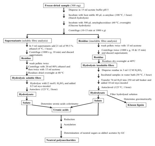
Figure 4. Simplified flowchart of the Uppsala Method used for determination of dietary fibre content (Theander *et al.*, 1995).
