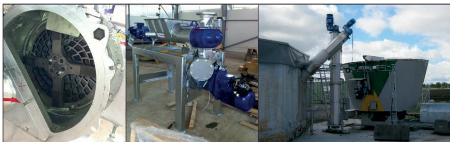
Figure 7. Equipment for pre-treatment and feeding of deep litter manure. Photo Karin Ahlberg Eliasson and Lars-Erik Jansson.
