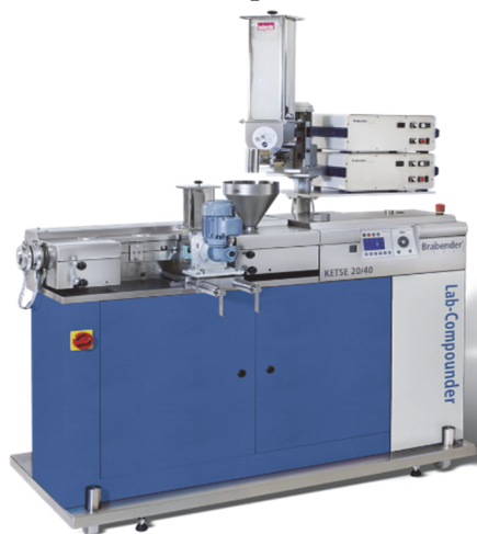
Figure 1 KETSE 20/40 extruder/ lab compounder.
