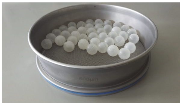
Figure 1 Sieving agitators (40 light and hollow plastic balls) as used on all test sieves finer than 1000 \mu\text{m}
