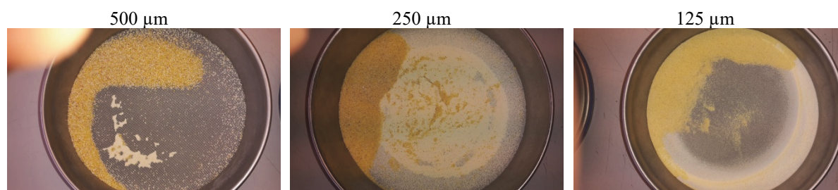
Figure 3 Agglomeration of maize meal on 500, 250, and 125 \mu\text{m} test sieves when no aids were used.
