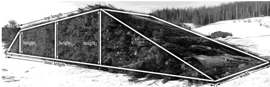
Figure 3. Dimension measurements on a windrow approximated as a trapezoidal prism.
