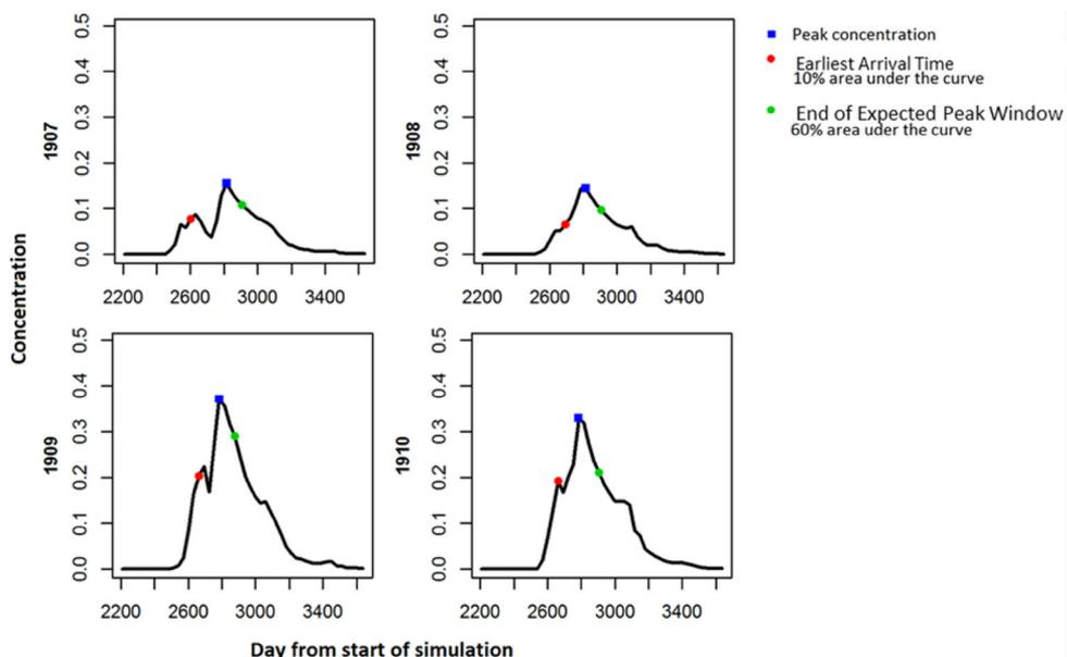
**Fig. 38** Example concentration time-series for a single application, illustrating how the earliest arrival time (10% of the area under the curve—AUC), expected peak window (10–60% AUC), and the months at target concentration (MTC) are defined
