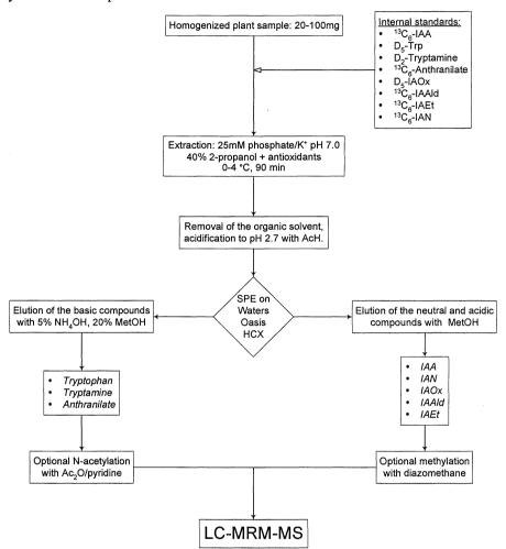
**Figure 10**: Sample preparation for IAA precursor analysis. Neutral/acidic and basic fractions from solid phase extraction (SPE) can either be combined and analysed together or analysed separately. All derivatization steps are optional, and the method was shown to work satisfactorily without them.
