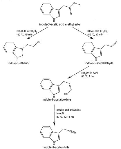
**Figure 9**: Chemical synthesis scheme of IAA metabolic precursors. Both [indole- $D_5$ ]- and [indole- $^{13}C_6$ ]-labelled IAA methyl esters were used for the synthesis
