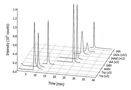
**Figure 11**: Example of the measurement of IAA precursors and related metabolites by LC-MRM-MS. Compounds (500 pg each) were separated by liquid chromatography and the reaction from the [MH<sup>+</sup>] to the most prominent daughter ion was monitored in MRM mode. Measurement groups used were based on retention time (see description in Paper VI).
