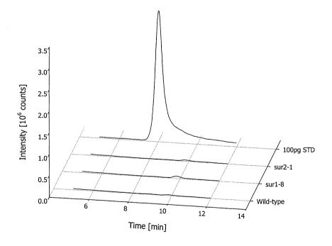
Figure 18: Tryptamine analysis in the wild-type and IAA overproducing mutants. The first three chromatograms represent transition from the  $[MH^+]$  ion at m/z 161 into the major daughter ion at m/z 144 (loss of ammonia, typical for primary amines in electrospray ionisation). The last chromatogram presents such transition for internal standard trace (m/z 163 into 146), and was taken from the wild-type sample (first chromatogram).
