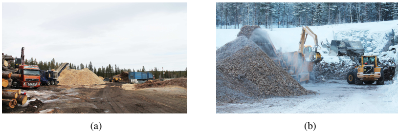
Figure 1.5: (a) Energy wood being loaded into a Petersson chipper by a truck-mounted crane (b) Stumps being loaded into CBI Magnum Force crusher by a grapple and front-end loader (Photos: Kalvis Kons).
