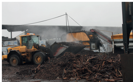
(a) Sawmill bark screening for energy with a mobile star screen at a terminal in northern Sweden (Photo: Kalvis Kons)
