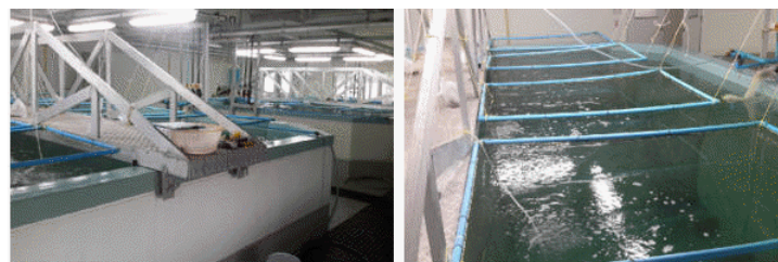
Figure 1. Experimental set up of experiment 1, with 16 hapas net divided equally between two 42 m 3 concrete tanks
