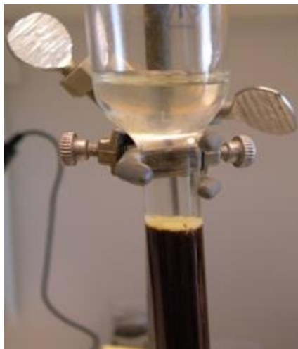
Figure 7. Resin in a column with white precipitates from the urine on top.
