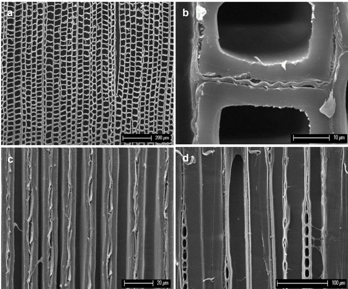
**Fig. 5.** SEM images of fresh spruce after MW irradiation. a) TS section showing a general loss of tracheid integrity and fractures in the ray canals; b) TS section of latewood tracheid showing modification of the compound middle lamellae between adjacent tracheids; c) RLS sections showing disruption of the middle lamella regions between axial tracheids; d) TLS section with ruptures in the middle lamellae regions between axial tracheids and ray/tracheid interphases
