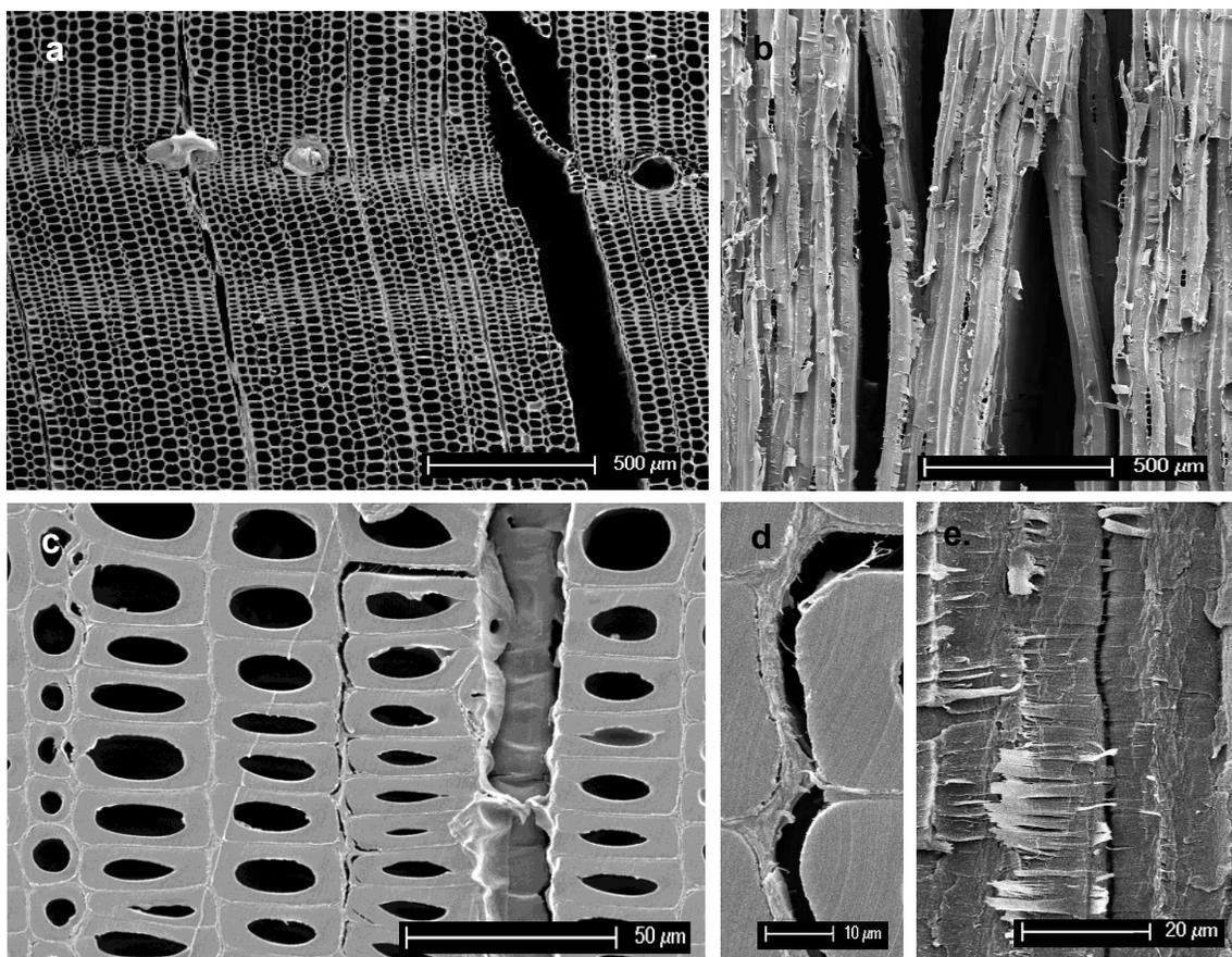
**Fig. 4.** SEM images of radiata pine after MW irradiation. a) TS section showing loss of tracheid integrity and fractures in ray canals; b) TLS section with longitudinal ruptures between separated tracheids; c, d) TS section of latewood with cracks formed along the radial and tangential walls of tracheids in middle lamella/primary wall regions; e) RLS showing ruptures along middle lamella/primary wall regions. Parts of the radial oriented  $S_1$  layer are also apparent
