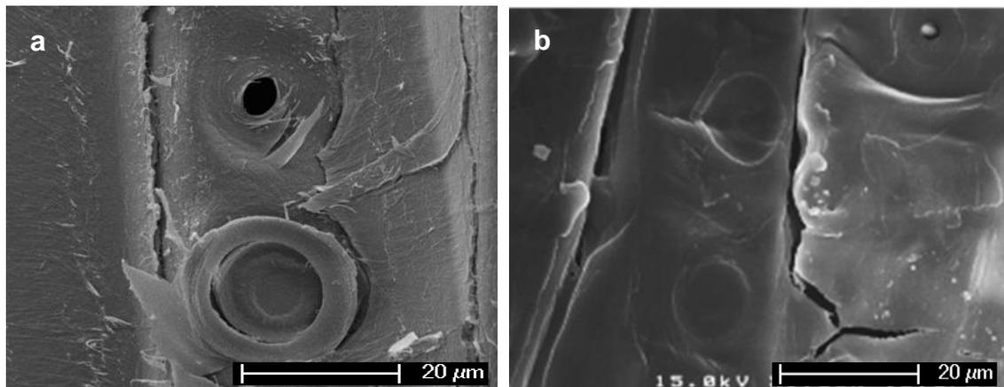
**Fig. 3.** Remains of pit apertures (left) after splitting and micro checks in S<sub>3</sub> cell wall of radiata pine earlywood tracheids treated by microwaves (right)
