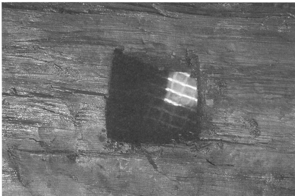
Fig. 25. Structural timber from a 1900 year old well. Detail showing the excellent preserved condition of the wood when wet. The hole for joining looks like it was manufactured yesterday and can successfully be recorded by the archaeologists. (Photo Anna Onsten)
