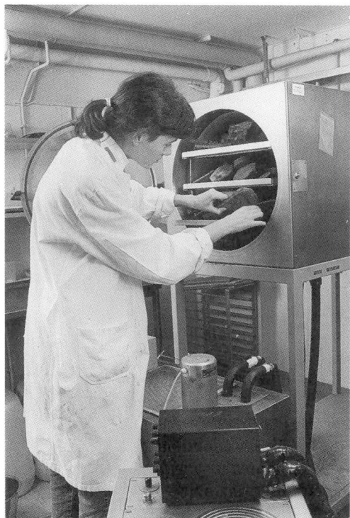
Fig. 26. Freeze-drying of archaeological wood samples at the Institute of Conservation, RAÄ, Sweden. In this type of conventional vacuum freeze-dryer, only smaller artefacts can be treated. (Photo Bengt Lundberg, RAÄ)
