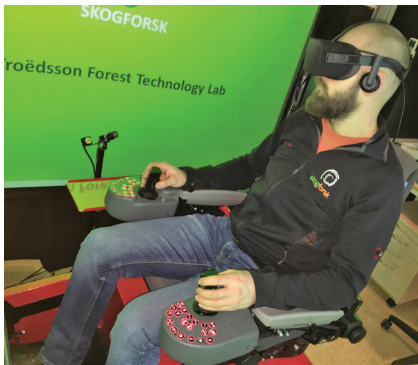
Figure 2. During the study, operators wore a virtual reality headset (brand Oculus Rift) which provided a 3-dimensional environment experience which is important during crane work. The Assortment Grapple does not require any special crane controls (i.e. joysticks), and standard controls, similar for all Nordic cut-to-length forwarders, are used
