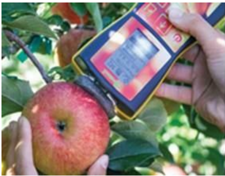
Figure 2 DA-meter measuring I_{AD} in 'Aroma'. Photo: I. Tahir
