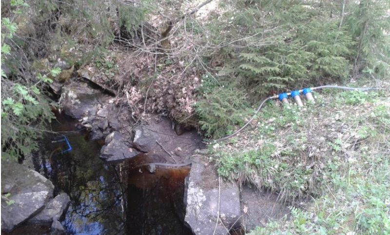
Figure 4. The source of the seeding community and carbon amendment for the growth medium. Water is being pumped out of the stream, through a series of filters, to the reverse osmosis machine (not shown).
