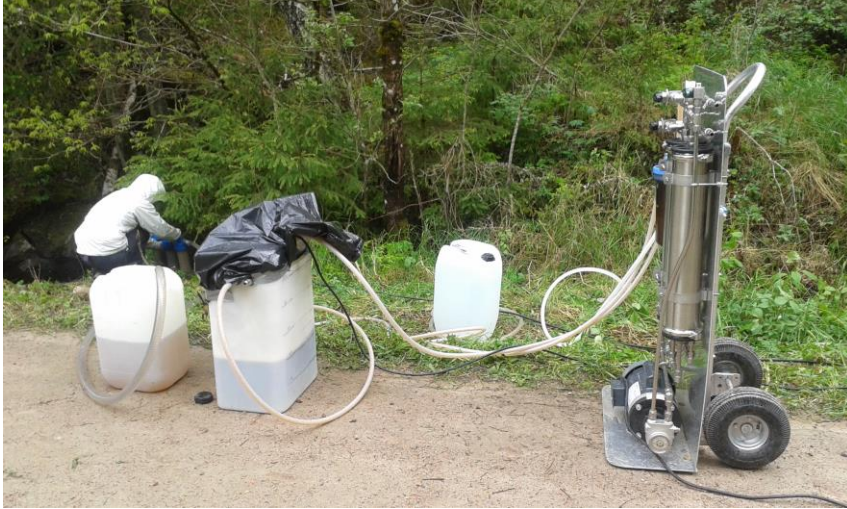
Figure 5. Portable reverse osmosis machine in action. This kind of machine is usually used for water purification. However, we discarded the ‘pure’ water permeate and collected the retentate (dissolved matter from the stream) into a bucket in order to concentrate it many times in order to facilitate transportation and storage of large quantities of natural dissolved organic matter for reproducible use in experiments.
