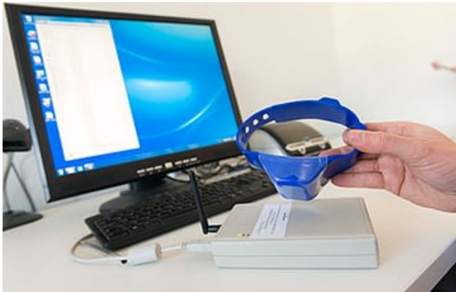
Figure 3. Data downloaded from an IceTag® sensor using the IceReader download station. Photo: www.icerobotics.com .
