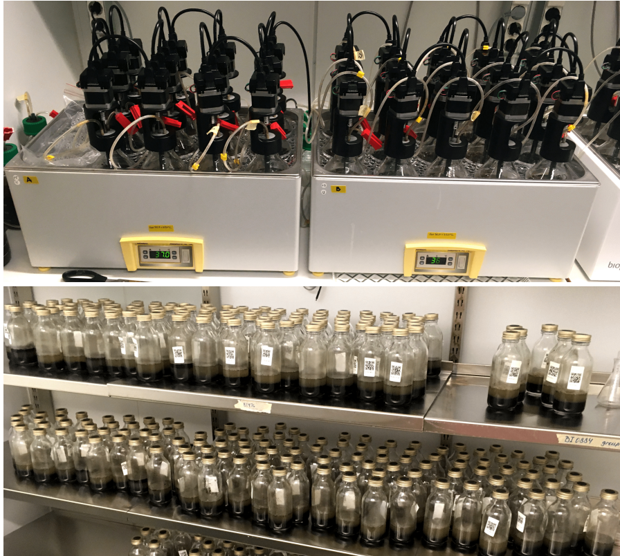
Figure 5: Biomethanation potential (BMP) is commonly measured either automatically using the automated AMPTS system (top), or manually using rubber-sealed bottles (bottom) .
