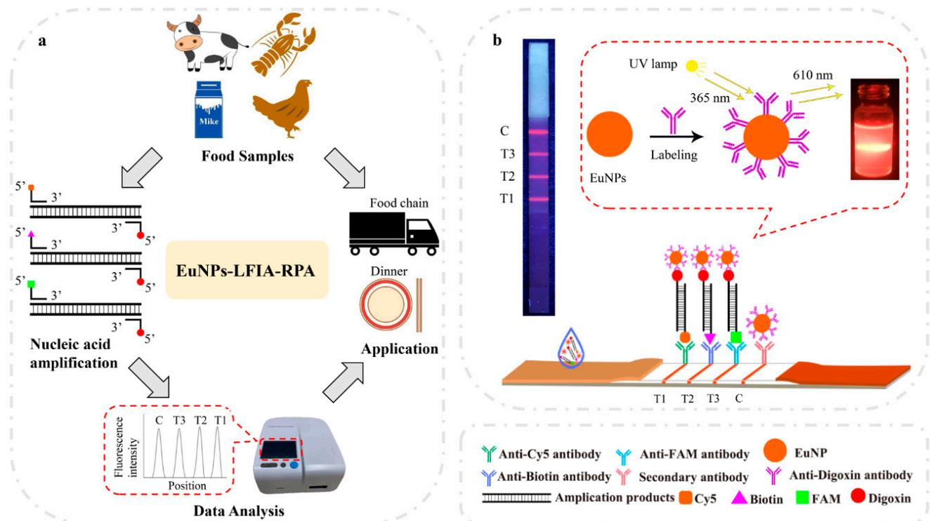
**Figure 1.** Schematic of EuNP-based LFIA–RPA. The application (a) and working principle (b) of the EuNP-based recombinase polymerase amplification combined with lateral flow immunoassay (EuNP-based LFIA–RPA).
