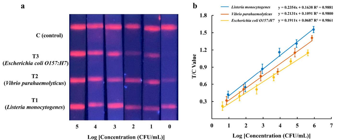
**Figure 3.** Reaction sensitivity of EuNP-based LFIA-RPA for *Listeria monocytogenes*, *Vibrio parahaemolyticus*, and *Escherichia coli* O157:H7. The amplified products could be observed using a portable 365 nm UV lamp (a). Standard curves for *Listeria monocytogenes*, *Vibrio parahaemolyticus*, and *Escherichia coli* O157:H7 (b).
