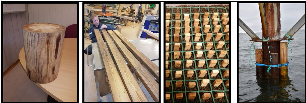
Figure 1. Treated wood pole (left), with 20cm diameter, treated wood boards with dimensions of 48x98mm (center), treated wood samples in soil contact according to EN 807 and wooden poles in marine tests(right).
