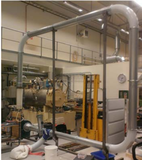
Figure 1: Closed loop apparatus used for the application of fire retardant and resin.
