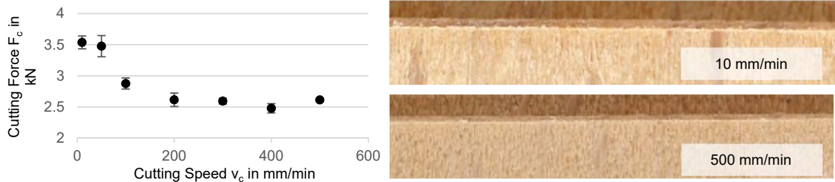
Figure 1. Influence of Cutting Velocity v_c on Cutting Force F_c ; Beech t_{BE} = 1,3 mm; \alpha_c = 90^\circ
