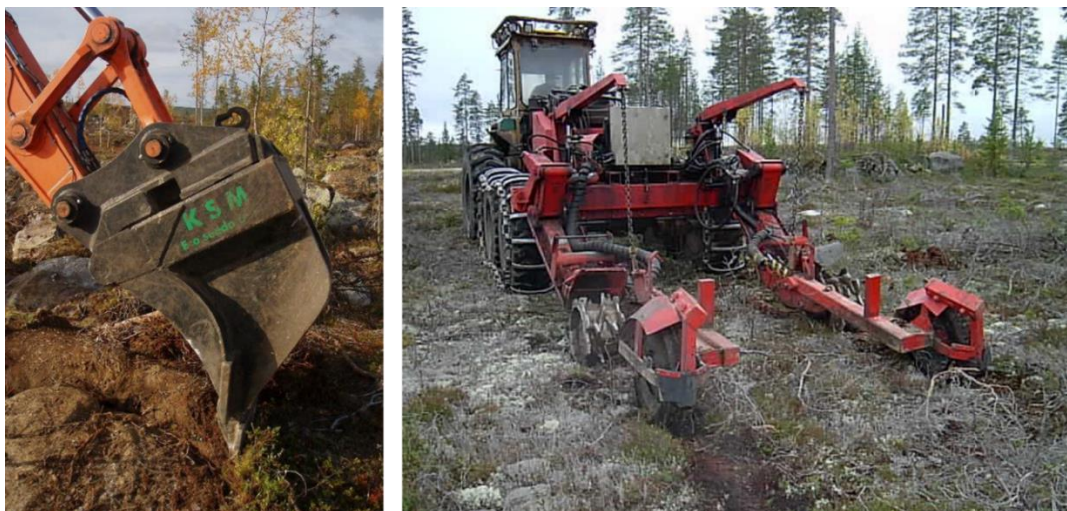
Figure 7. Examples of specifically designed devices for mechanized direct seeding: the KSM bucket (a crane/boom-mounted seeding bucket, left) on an excavator for direct seeding in patches; the HuMinMix (Humus Mineral soil Mix, right) mounted on a forwarder for continuously advancing row seeding in rototilled, micro-prepared, shallow trenches. Photo: Ida Nilsson and Tomas Nordfjell.
