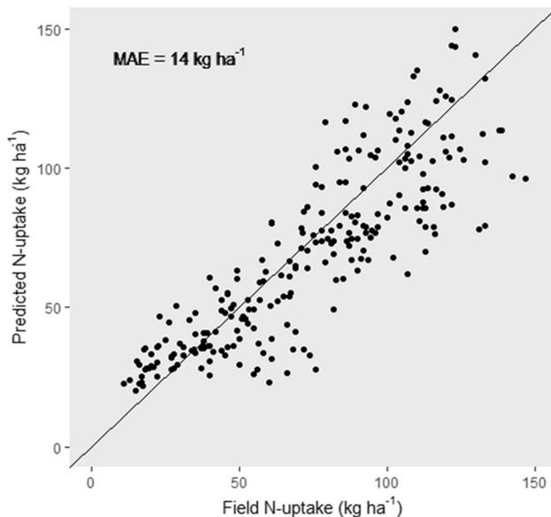
**Fig. 6** Spatiotemporal cross-validation prediction based on a chlorophyll index (CI) model for top of atmosphere (L1C) satellite data versus field nitrogen (N)-uptake obtained from the proximal canopy reflectance sensor. The mean absolute error (MAE) is also shown
