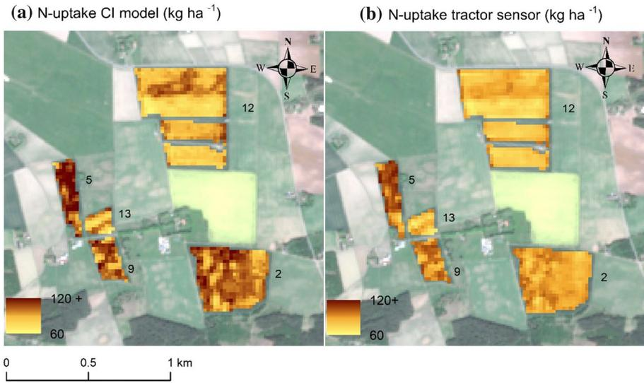
**Fig. 11** Close-up view of some of the Ardala fields (location in Fig. 1). Left: the nitrogen (N)-uptake calculated from the satellite prediction model. Right: Interpolated N-uptake data from the tractor-borne N-sensor within two days of the acquisition date of the satellite image. The different fields are labelled with their field identification (ID) number (cf. Table 3; Fig. 10). Background: Sentinel-2 true colour composite with sensing date 27 May, 2017
