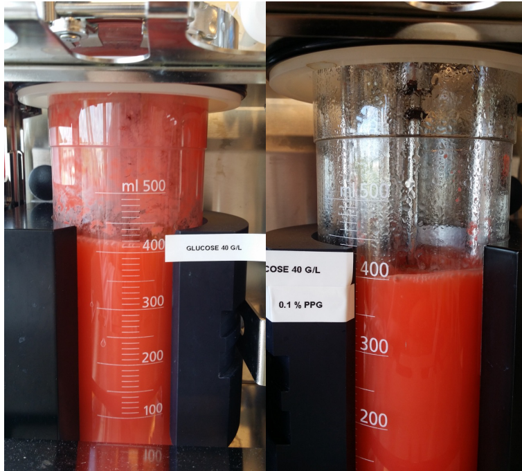
Figure 13. Cultivation of R. toruloides CBS14 using 0.1% PPG volume. Using PPG prevented yeast adhesion to vessel.
