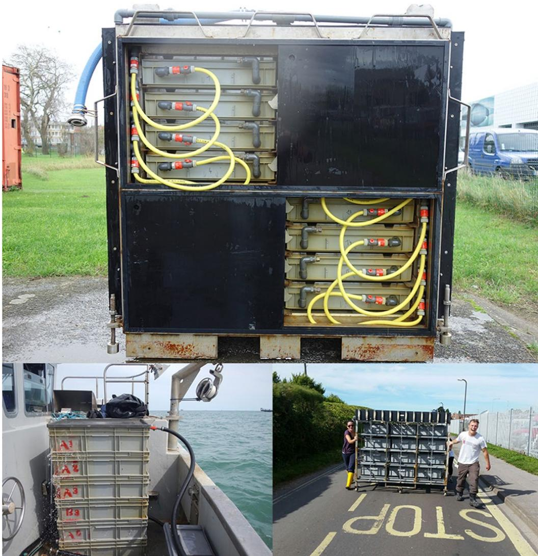
Figure 9.4. Top: on-board monitoring rack (152 cm L × 59 cm W × 160 cm H) with 16 independently-mounted, flow-through, 30-l monitoring containers (60 cm L × 40 cm W × 12 cm H). [Credit: Flanders research institute for agricultural, fisheries and food research (ILVO)]. Bottom: similar racks used in the UK [Credit: Centre for environment, fisheries and aquaculture science (Cefas)].
