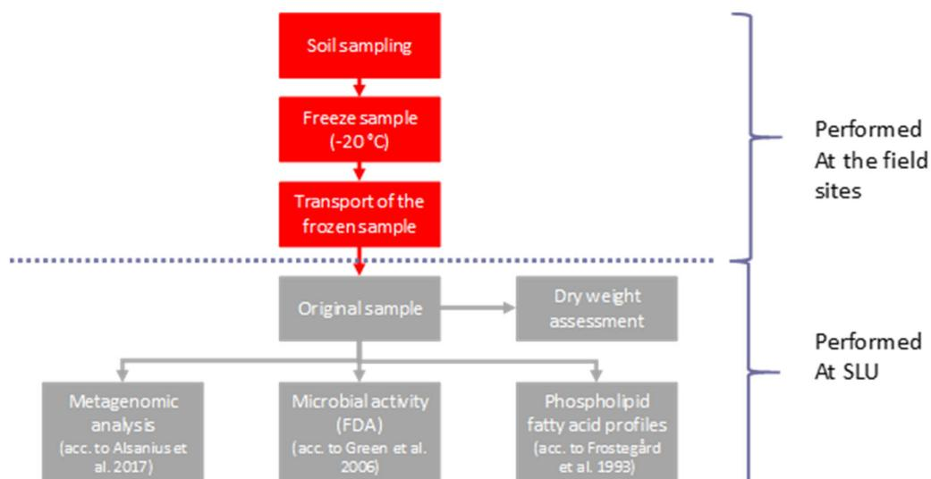
Figure 4 Flow chart of soil samplings and analyses
