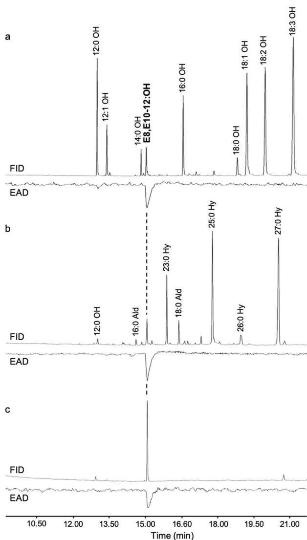
Fig. 11 Gas chromatographic analysis of plant and insect derived pheromone and synthetic pheromone simultaneously using a flame ionization detector (FID) and a male C. pomonella antennae as an electroantennographic detector (EAD). a Alcohol products converted from seed oil fatty acids of a stably transformed C. sativa line expressing a thioesterase and a desaturase ( Cpo_CPRQ ) elicit an antennal response at the retention time corresponding to the pheromone component ( E,E )-8,10-dodecadienol (E8,E10-12:OH); b antennal response to the female pheromone gland extract (1/5 female equivalent); c antennal response to the synthetic codlemone
