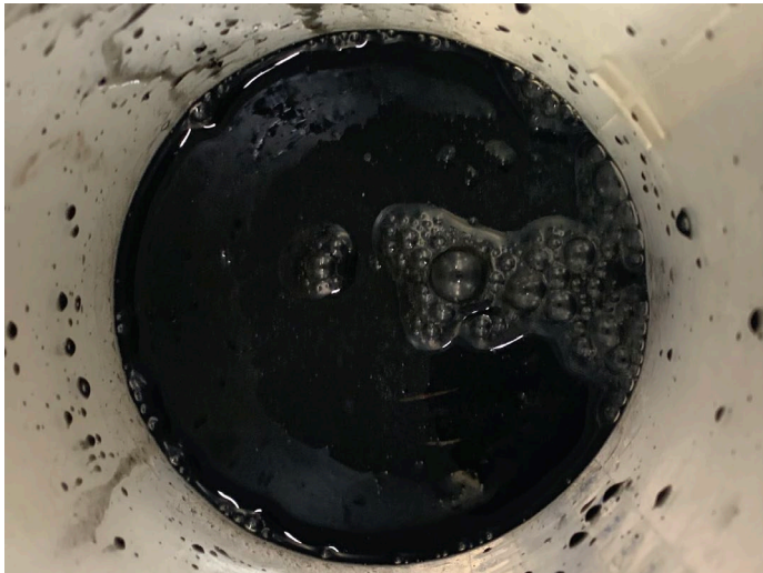
Figure 6. Biogas digestate from a laboratory-scale reactor processing food waste.
