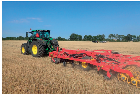
Figures 19. Tractor and cultivator at work (a) with specially equipped towing eye (b) at working depth of 12 cm (c) with cultivator discs lifted (d). Photo: Jens Blomquist.
