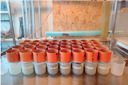
Figure 10. After shallow tillage, the loose soil was sieved into three size classes (a). Aggregates 2-5 mm (b) were sampled and transported in plastic jars (c) to the Swedish University of Agricultural Sciences (SLU) in Uppsala. After drying, the aggregates were subjected to two simulated rainfall events 24 hours apart (d). The leachate (in transparent plastic jars below the orange plastic pipes containing the aggregates) was collected after each rainfall event (e). Turbidity was measured in leachate after each simulated rainfall event. Turbidity and electrical conductivity (EC) were determined (f). Turbidity indicates clay dispersion of the aggregates and is therefore an indicator of aggregate stability and a proxy for the risk of particulate phosphorus (PP) losses. Photo: Jens Blomquist.
