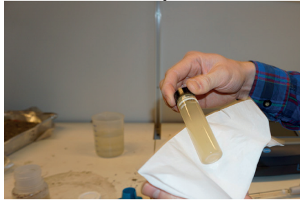
Figure 10. After shallow tillage, the loose soil was sieved into three size classes (a). Aggregates 2-5 mm (b) were sampled and transported in plastic jars (c) to the Swedish University of Agricultural Sciences (SLU) in Uppsala. After drying, the aggregates were subjected to two simulated rainfall events 24 hours apart (d). The leachate (in transparent plastic jars below the orange plastic pipes containing the aggregates) was collected after each rainfall event (e). Turbidity was measured in leachate after each simulated rainfall event. Turbidity and electrical conductivity (EC) were determined (f). Turbidity indicates clay dispersion of the aggregates and is therefore an indicator of aggregate stability and a proxy for the risk of particulate phosphorus (PP) losses. Photo: Jens Blomquist.
