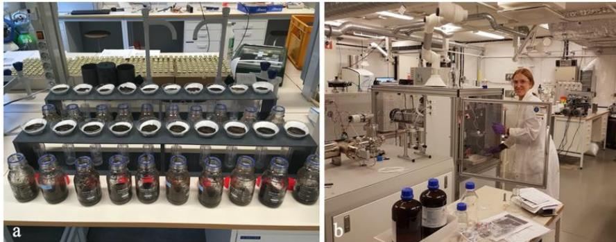
**Figure 10.** KCl extraction and filtration of mineral soil samples that have been isotopically labeled with <sup>15</sup>N (a). Adjustments of the SPINMAS instrument used for analyzing gross N transformation rates (b). Photos: Theresa S. Ibáñez (a), Gabriel Ibáñez (b).
