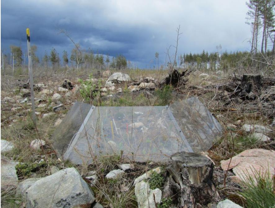
**Figure 1.** A low fire severity salvage logged site, with an open top chamber (OTC) positioned to test experimental warming on boreal forest tree seedling growth, studied in paper III. Photo: Theresa S. Ibáñez.
