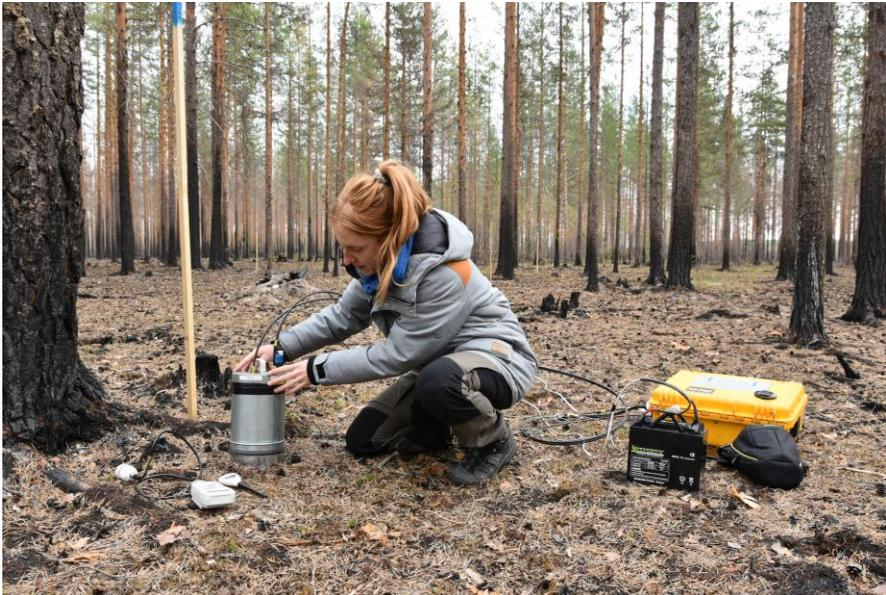
**Figure 7.** Soil respiration measurements with an Ultraportable greenhouse gas analyzer (UGGA) in a high fire severity stand in the Ljusdal fire area (paper IV). Photo: Natascha Kljun.
