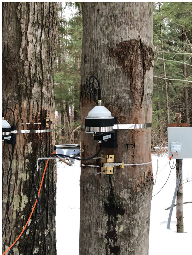
Fig. 1. Examples of an automatic band dendrometer (upper instrument on tree) co-located with an automatic point dendrometer band (middle left on tree) and standard manual band dendrometer (lowest instrument on tree) at the Hubbard Brook Experimental Forest, N.H., USA (photograph by L.E. Rustad).
