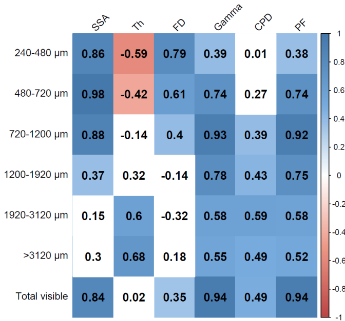
Figure 10. Correlation matrix of X-ray derived pore size distributions and macropore network characteristics. Significant correlations ( P < 0.05 ) were highlighted either in red (negative) or in blue (positive). SSA: specific surface area of macropores, Th: average macropore thickness, FD: surface fractal dimension, Gamma: connection probability, CPD: critical pore diameter, PF: percolating fraction.
