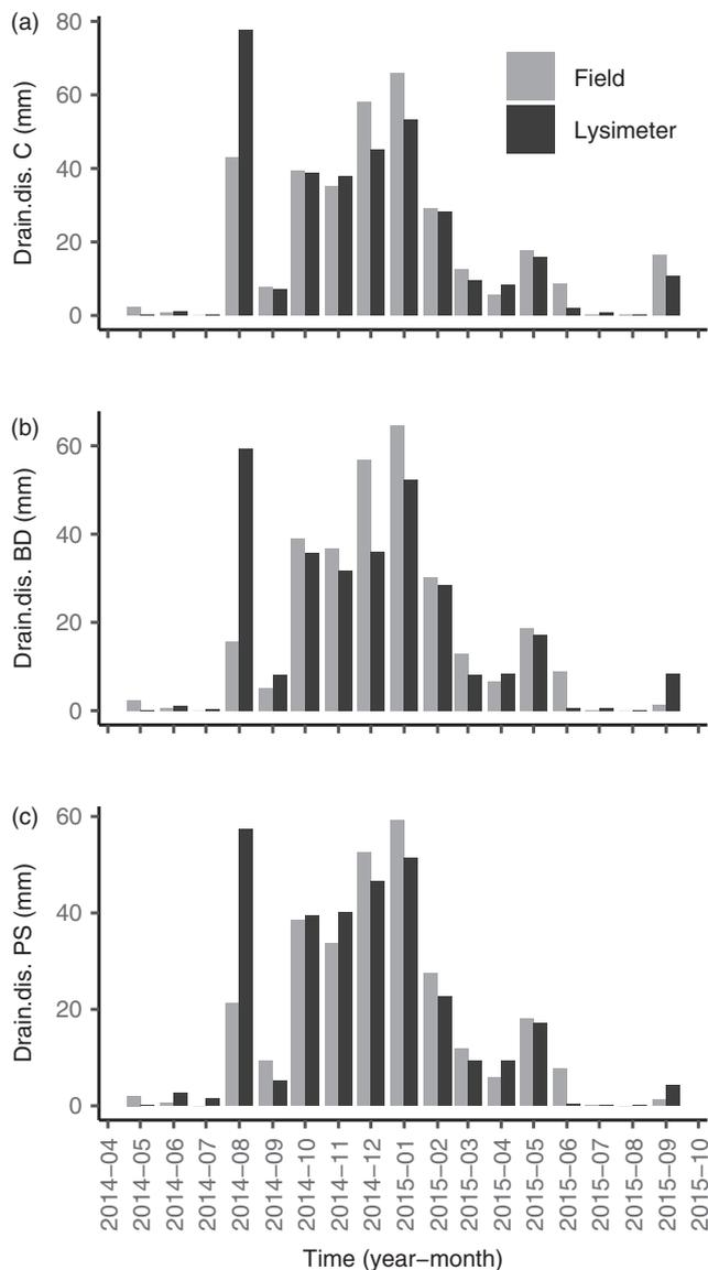
**FIGURE 5** Drainage discharge (drain. dis.) per month, as treatment means, in the field and in the lysimeters, 20 May 2014–16 September 2015. (a) Control (C), (b) biogas digestate (BD) and (c) pig slurry (PS) treatments. Note different scale on the y-axes in (a), (b) and (c)
