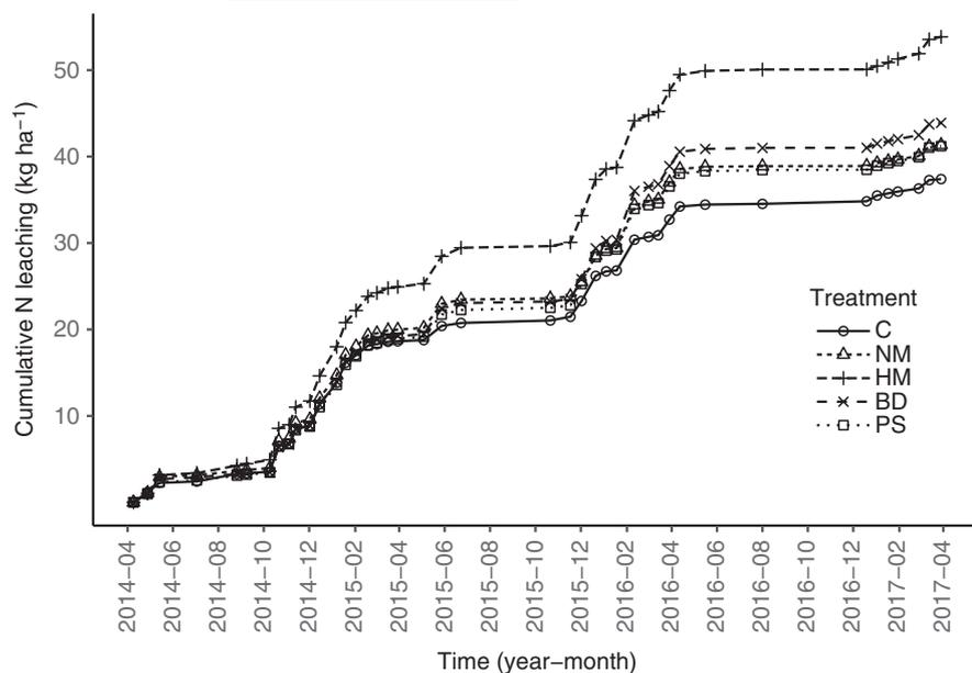
**FIGURE 4** Cumulative nitrogen (N) leaching in the tile-drained field from April 2014 to March 2017, as treatment means. Treatments: BD, biogas digestate; C, control; HM, high mineral N; NM, normal mineral N; PS, pig slurry
