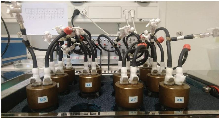
Figure 10. The set-up of the *in vitro* gas production experiment in one of three water baths (Paper I). Bottles containing feed samples and buffered rumen fluid are submerged in a water bath and the bottles are connected with tubes to gas recording boxes.
