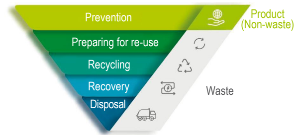
Figure 1. The waste hierarchy dictating how waste should be treated in the European Union.
